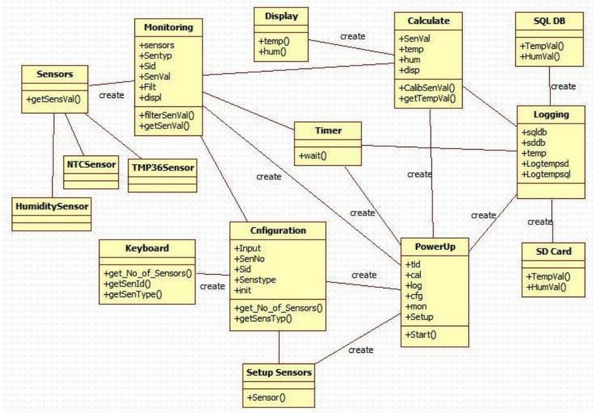
Figure 0-10: Object Diagram for the Home Automation System
