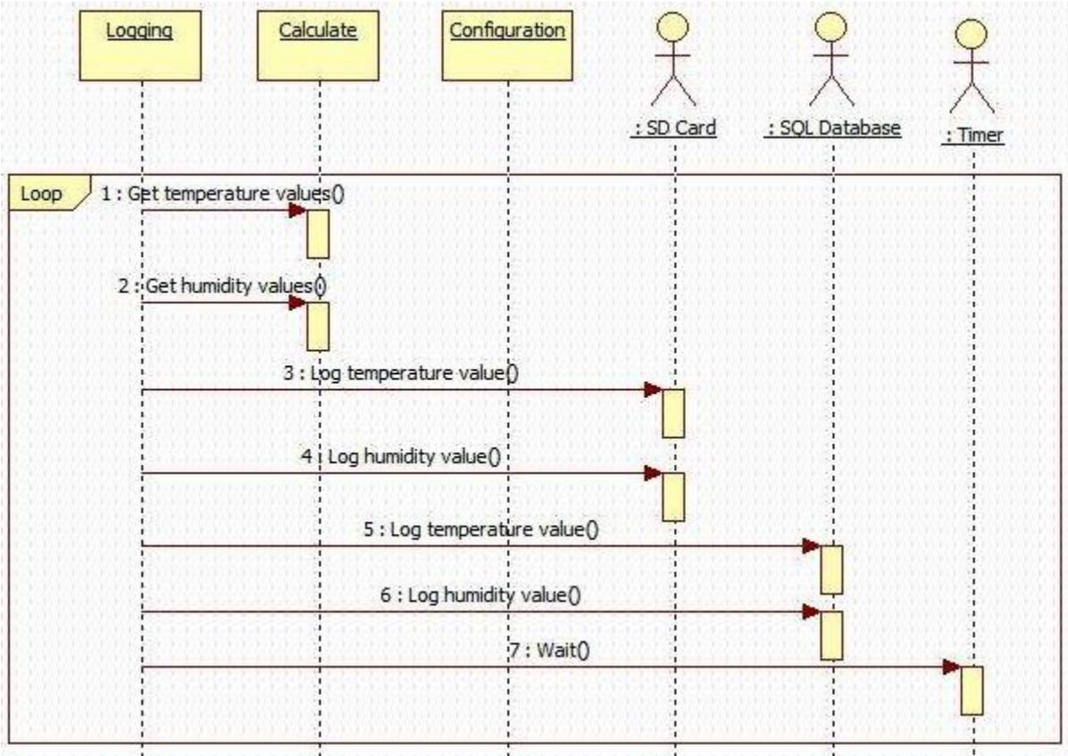
Figure 0-1: System Sequence Diagram (SSD) for 'Logging' Use Case Diagram
