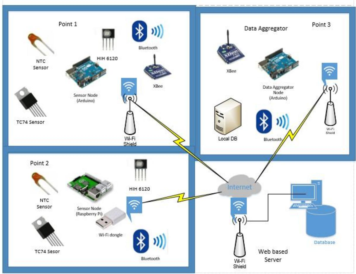
Figure 2-3: Different Wireless Means of Communication between the Sensor Nodes (point 1 and point 2) and the data Aggregator
