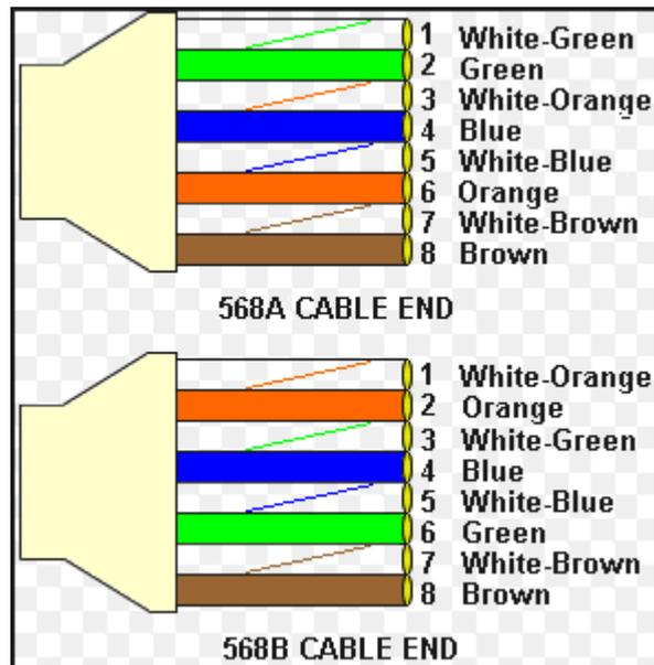
Figure 2-2: Color Codes for the Twisted Pair Ethernet Cable [17]
