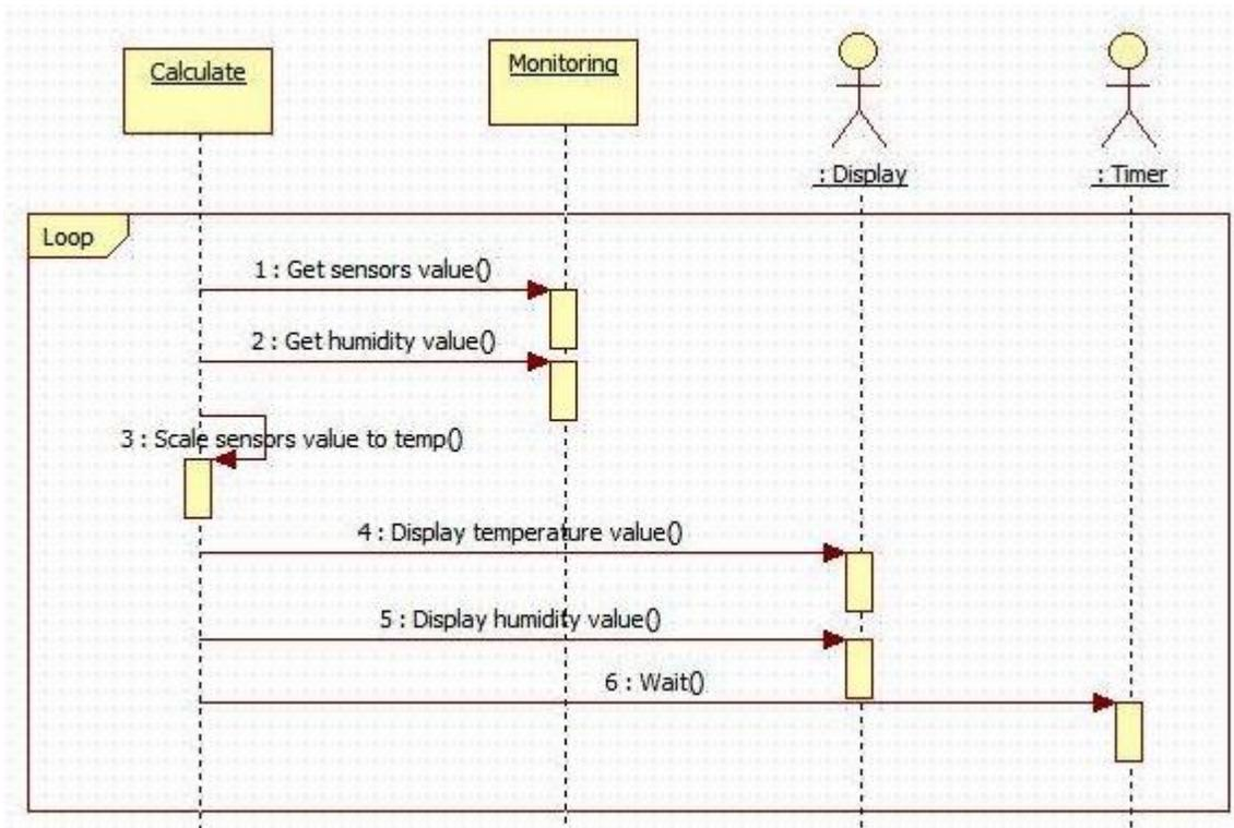
Figure 0-3: System Sequence Diagram (SSD) for 'Calculate' Use Case Diagram
