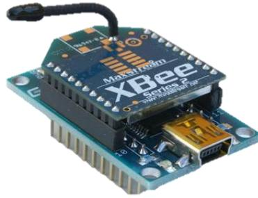
*Figure 1-8: XBEE module mounted on Adapter board*
