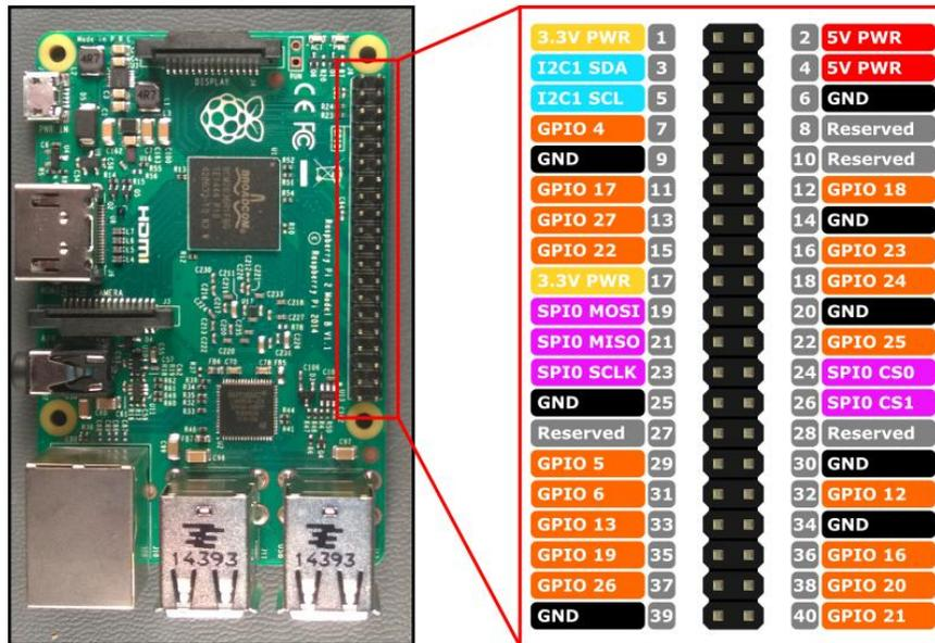
Figure 1-7: Pinout of Raspberry Pi 2 [10]
