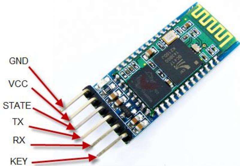
*Figure 1-11: HC-05 Bluetooth Module with pin assignment*
