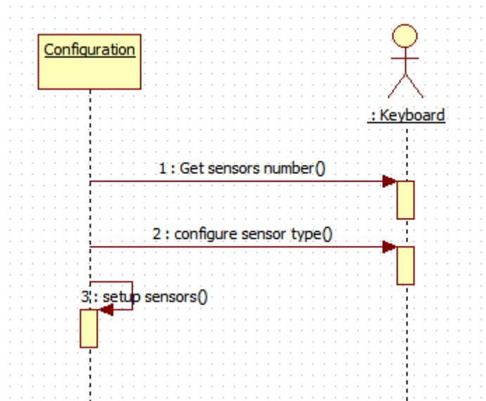
Figure 0-4: System Sequence Diagram (SSD) for 'Configuration' Use Case Diagram
