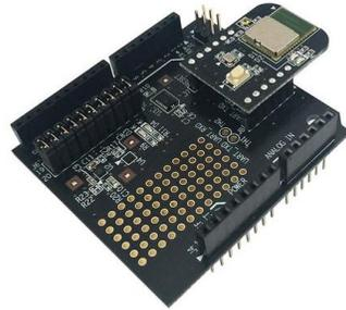
*Figure 1-10: Bluetooth Smart Shield mounted on Arduino Bluetooth Shield*
