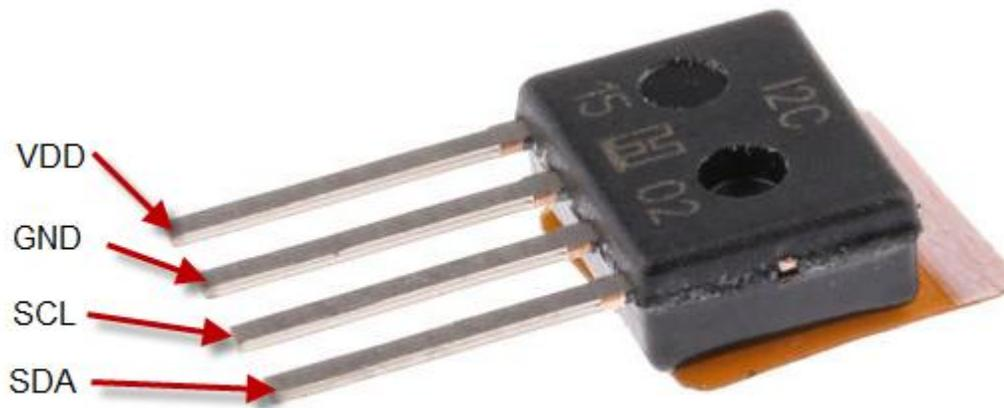
*Figure 1-14: HIH-6120 Temperature and Humidity*
