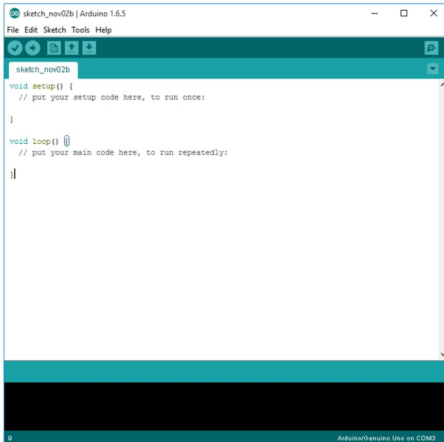
*Figure 1-5: Screen shot of Arduino IDE*
