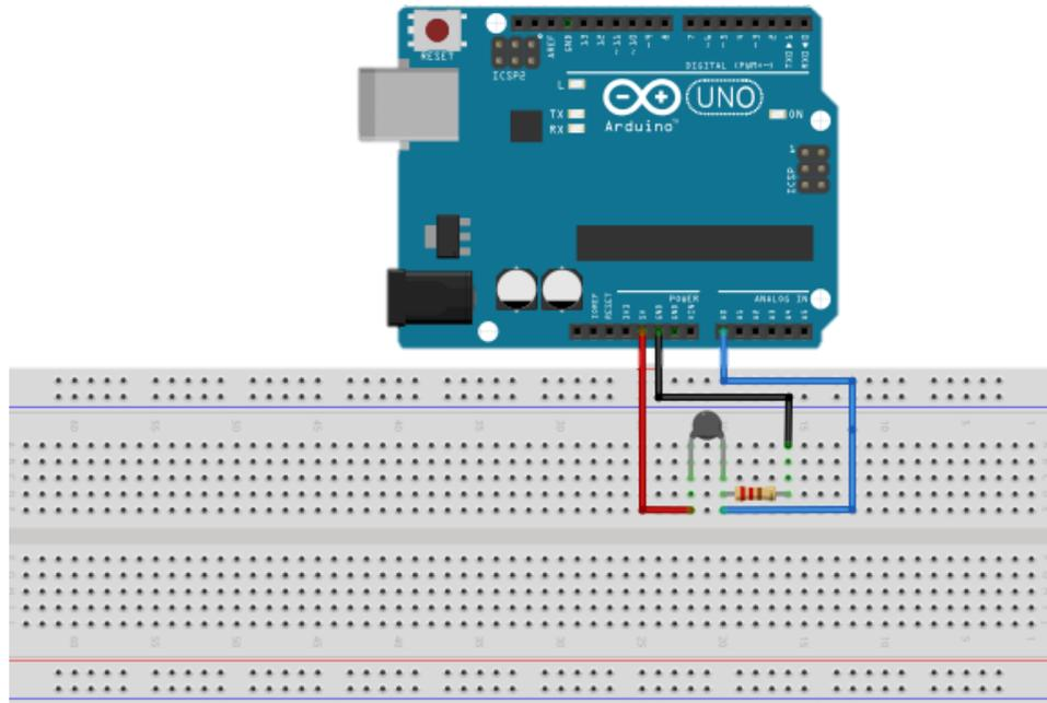
Figure 4-2: NTC Temperature Sensor Connection to Arduino Board
