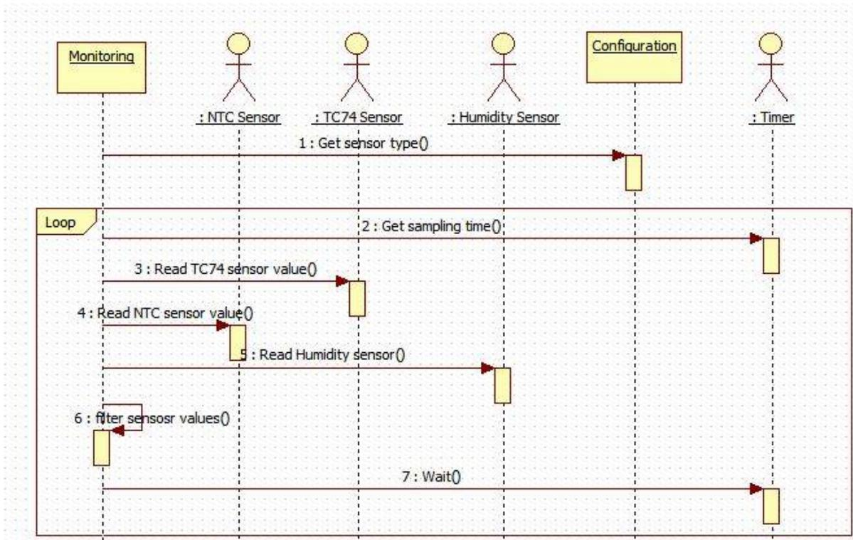
Figure 0-2: System Sequence Diagram (SSD) for 'Monitoring' Use Case Diagram
