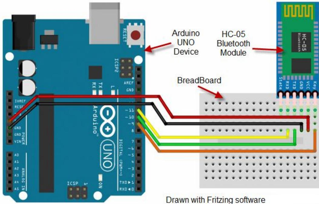
*Figure 4-8: Connection of HC-05 with Arduino UNO device*
