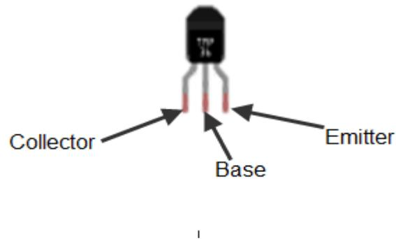
*Figure 1-12: TMP36 Temperature Sensor*
